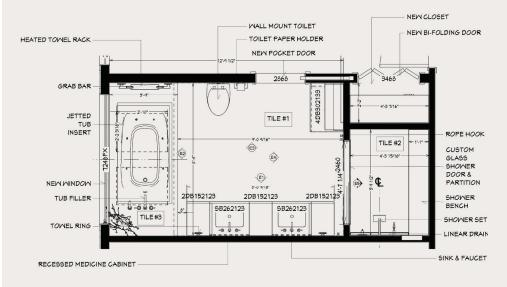
By taking 60 square feet from the former walk-in closet, the designers were able to fit in a bathtub; they relocated all the fixtures to reserve the area by the window for this tub.
